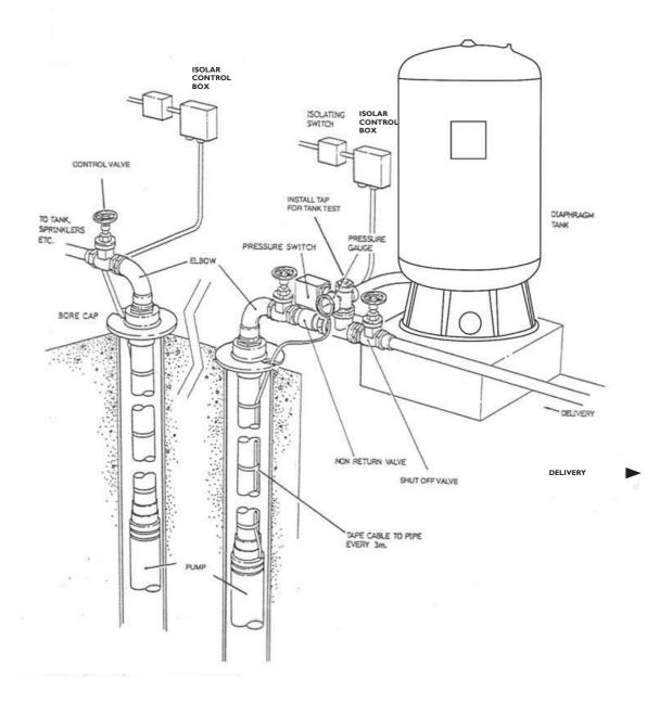
Pump connected for manual operation
